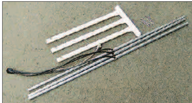
Figure 5 — The triangle HPOD disassembled for transport.
